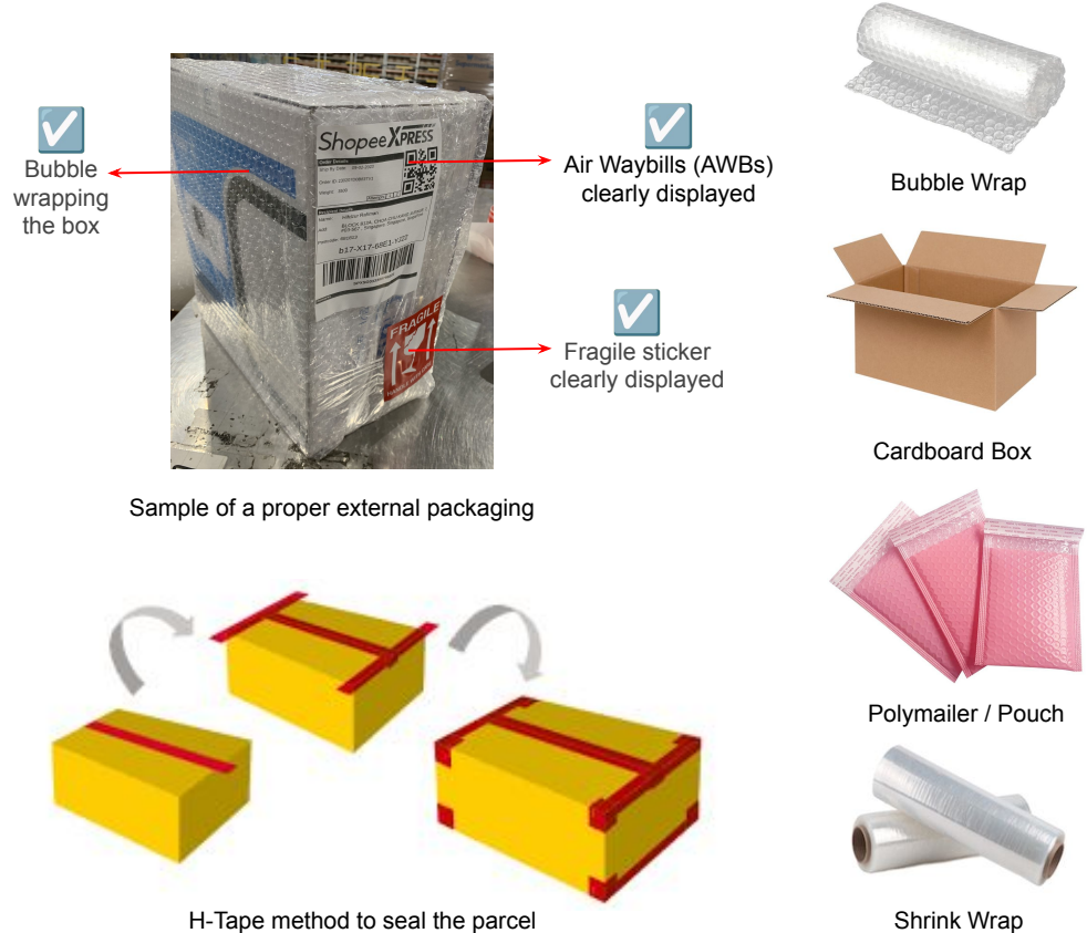
H-Tape method to seal the parcel
